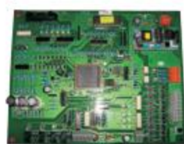
日立电梯门机板 DMC-1 SP1210 HITACHI elevator Gantry crane board DMC-1
