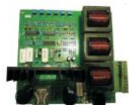
门机调速板 Door Machine speed regulation PCB XDMJ-TS110 sp4692
