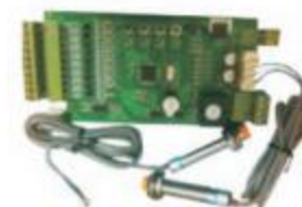
扶梯防逆转装置 Escalator deflector PCB sp4812
